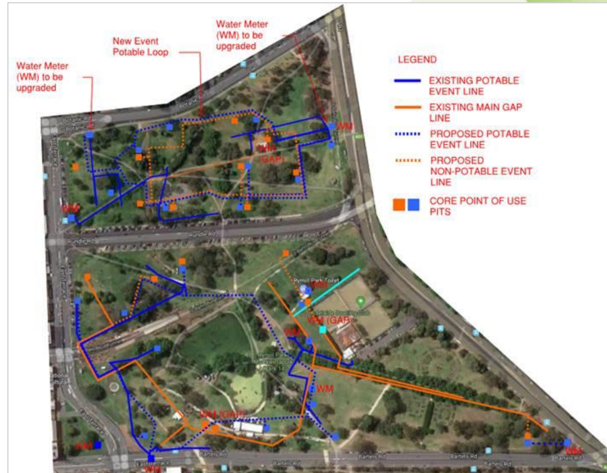
Expanded Recycled Water Access Site Map for Event Infrastructure Project at Rundle and Rymill Parks
